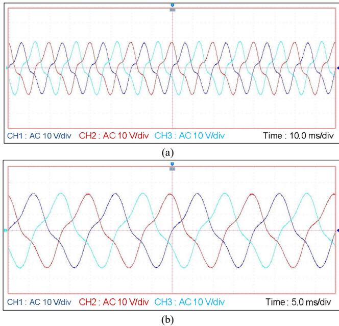
Fig. 12 The experimental results. (a) stator voltage at wind speed 6 m/sec, (b) stator voltage at wind speed 9 m/sec
