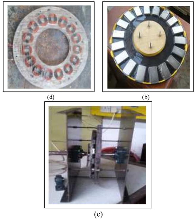
Fig. 7 The manufacturing of AFDPMMSG. (a) stator disc, (b) rotor disc (c) Assembled result
