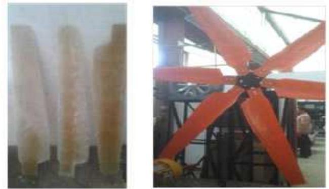
Fig. 4 The HAWT manufacturing results.
