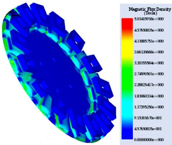
Fig. 6 The magnetic flux density of the AFDPMMSG rotor
