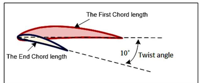
Fig. 2 The blade airfoil
