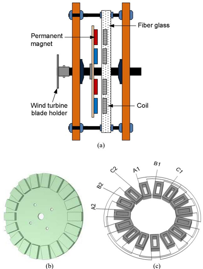
Fig. 5 The design of AFDPMMSG. (a) the structure of AFDPMMSG, (b) rotor disc, (c) stator disc
