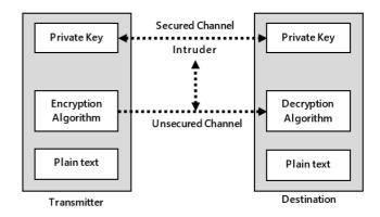
Fig. 1 General Construction of Symmetric Encryption Algorithms.
