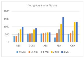
Fig. 4 Decryption time vs. file size for DES, 3DES AES, RSA and OtO
