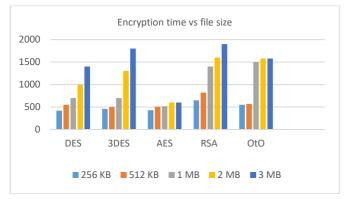
Fig. 3 Encryption time vs file size for DES, 3DES AES, RSA and OtO
