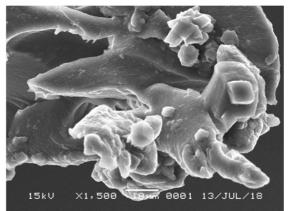
Fig. 10 SEM test result of a cross-section from membrane Pec-Chi-BADGE  $% \mathcal{A}$
