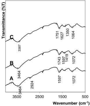
Fig. 11 FTIR test result from membrane: A. Chitosan; B. Pectin; C. Pectin-Chitosan-BADGE
