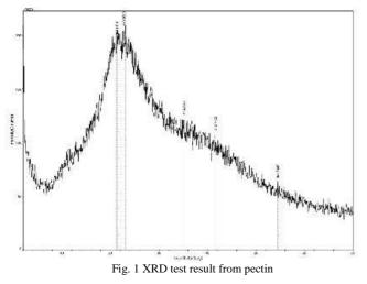
It has one broad, sharp peak only at an angle  $(2\Theta) = 21^{\circ}$  degree whereas chitosan (Figure 2) is semi-crystalline because it has the height at an edge  $(2\Theta)$  of  $11^{\circ}$  and  $21^{\circ}$ . If we look, Pec-Chi-BADGE (Figure 3) adsorbent shows no peak in the XRD pattern.
