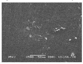
Fig. 6 SEM test result of the surface from membrane chitosan
