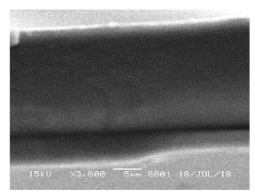
Fig. 8 SEM test result of a cross-section from membrane pectin
