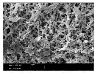
Fig. 6 SEM of the MIP endosulfan template at 1.99 KX magnification and 30  $\mu m$  resolution
