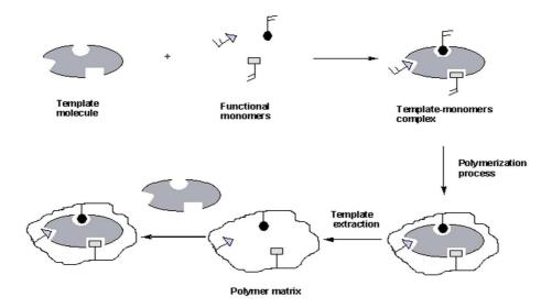
Fig. 2 Scheme of molecular imprinting
