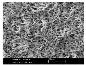
Fig. 3 SEM of the MIP endosulfan template at 500X magnification and 30 um resolution
