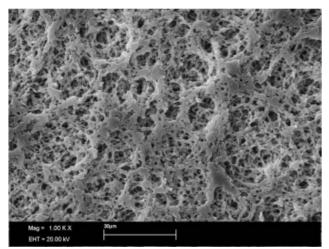
Fig. 4 SEM of the MIP endosulfan template at 1.0 KX magnification and 30  $\mu m$  resolution
