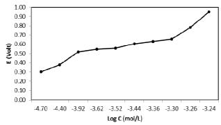
Fig. 12 Graph of MIP potential of endosulfan to the target of logarithm concentration on the aluminum-carbon electrodes on at  $20^{\rm th}$  day
