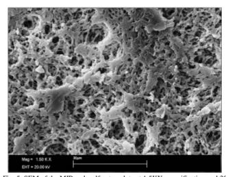
Fig. 5 SEM of the MIP endosulfan template at 1.5KX magnification and 30  $\mu m$  resolution
