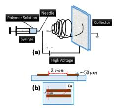
Fig. 1. Schematic diagram of (a) electrospinning system and (b) substrate with a patterned electrode
