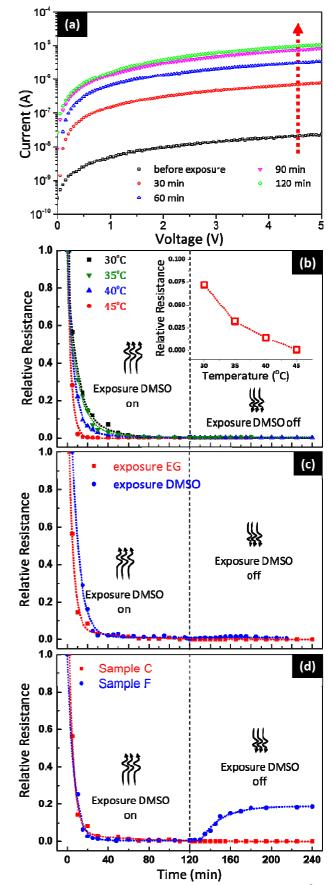
Fig. 6. (a) I-V Characteristics of sample C exposure DMSO at 40  $^{\circ}$ C, (b) relative resistance of sample C exposure DMSO various temperature (insert relative resistance vs temperature at min 40), (c) sample C with various exposure solvent at 40  $^{\circ}$ C, (d) sample C and F exposure DMSO at 40  $^{\circ}$ C.
