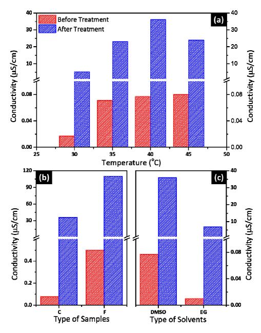
Fig. 7. Summary of conductivity improvement of (a) sample C with various DMSO temperatures, (b) Type of sample exposure DMSO at 40  $^{\circ}$ C, and (c) sample C with a different type of solvent used.
