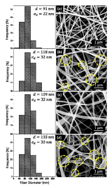
Fig. 4. SEM image and nanofiber diameter distribution, (a) sample C before, (b) after exposure DMSO at 40 °C for 2h; (c) sample F before, (d) after exposure DMSO at 40 °C for 2h
