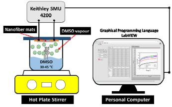
Fig. 2. Schematic diagram of solvent vapour treatment and electrical conductivity measurement.
