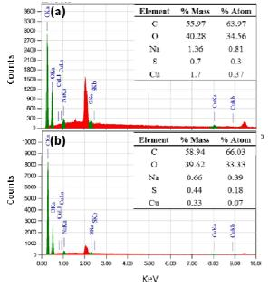
Fig. 5. EDS result of sample C (a) before, (b) after exposure DMSO for 2 h at temperature 40  $^{\circ}\text{C}$
