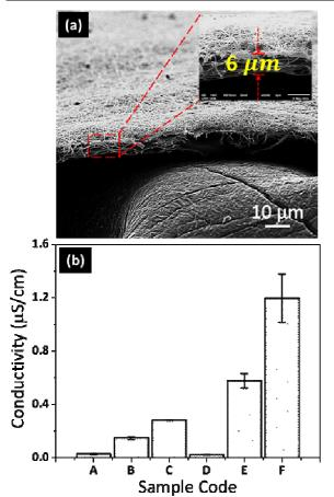
Fig. 3. (a) SEM image of cross-section of sample C; (b) conductivity of samples
