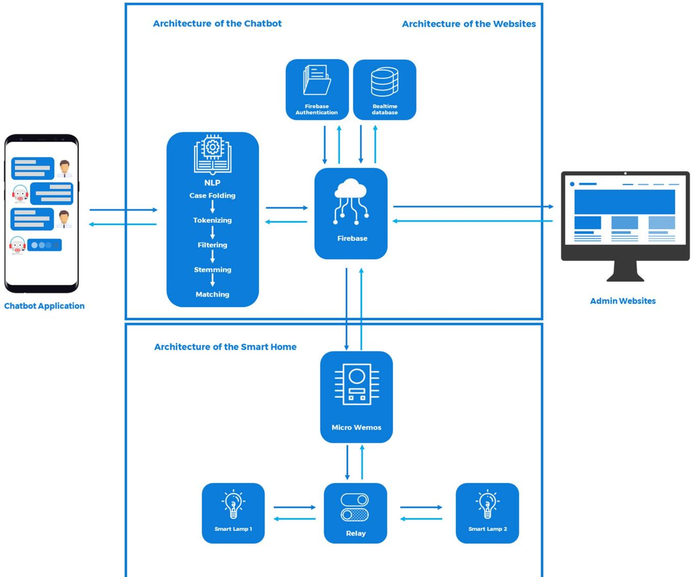
Fig 1. The proposed system architecture
