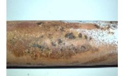
Fig. 3 As-received tube showing the tube pitting corrosion
