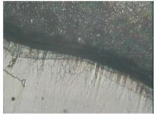
Fig. 7 Photomicrograph showing DMW creep voids at ferritic interface
