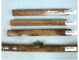
Fig. 1 The as-received failed high temperature superheater (HTS) tubes
