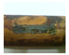
Fig. 2 Close view of failed HTS tubes
