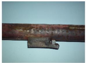
Fig. 8 General view of welding between superheater tube and support-clip
