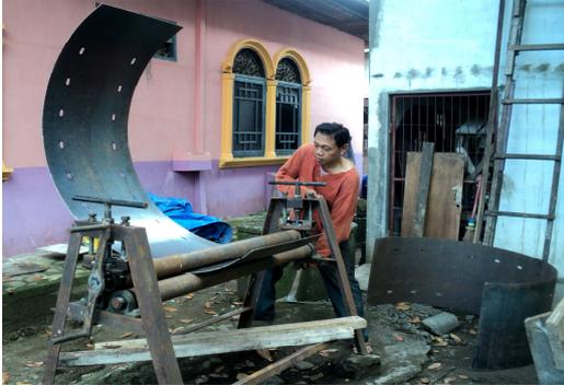
Fig. 9 The process of rolling inner rings a water wheel
