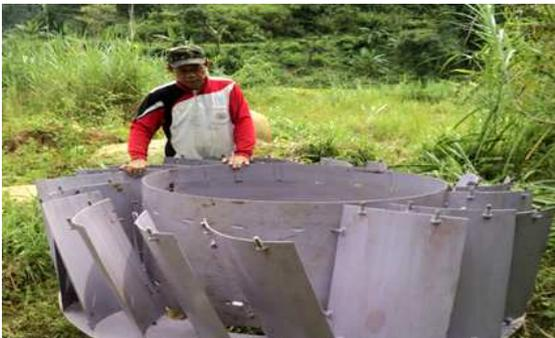
Fig. 11 installation of 20 blades in the water wheel main ring
