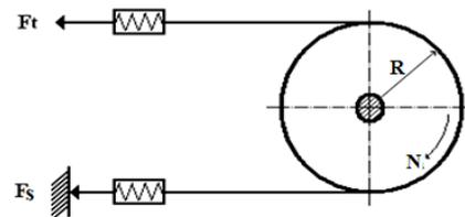
Fig. 15 W2KDS torque measurement scheme
