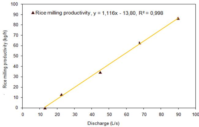
Fig. 22 Rice milling productivity versus discharge
