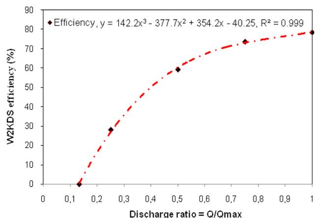
Fig. 19 Variation in the efficiency W2KDS versus discharge ratios
