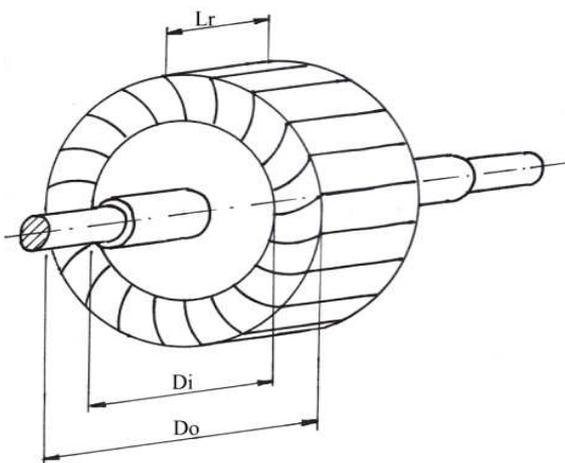
Fig. 7 The main dimensions of the wheel
