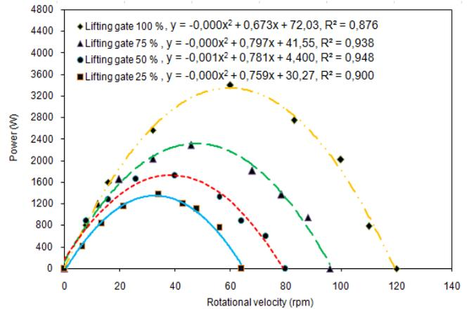
Fig. 16 Curve effect of rotational variations on W2KDS power
