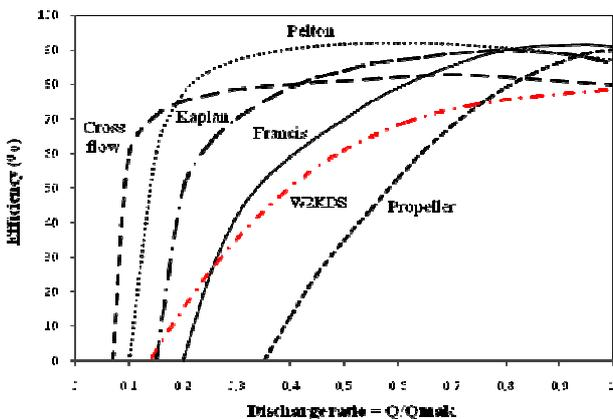
Fig. 20 Trend of efficiency versus discharge ratio of five conventional turbines compared to W2KDS
