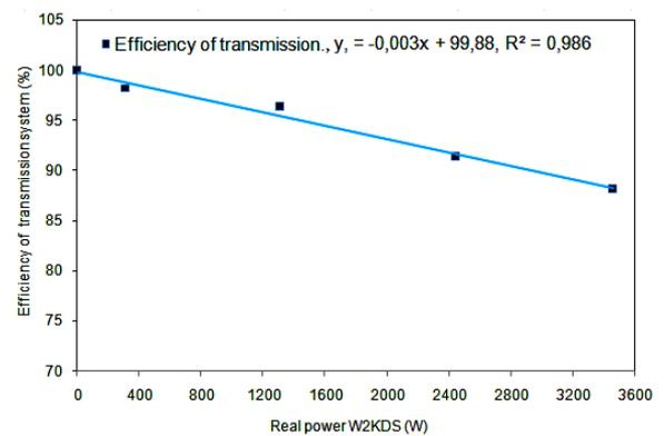
Fig. 21 Variation in the efficiency of transmission of real power
