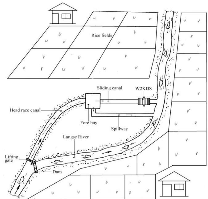
Fig. 5 Layout around the W2KDS testing location
