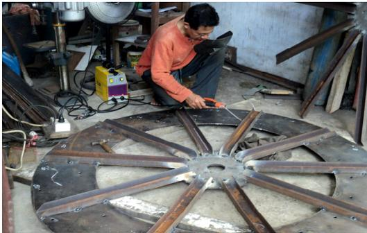
Fig.10 the process of making the water wheel main ring
