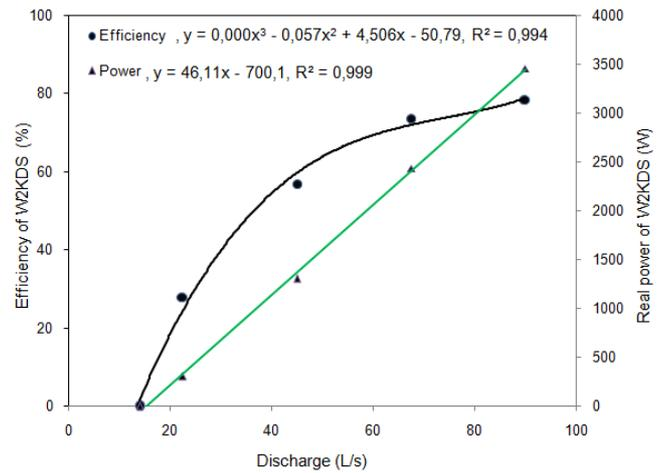
Fig. 18 Variation in the efficiency and real power of W2KDS versus discharge
