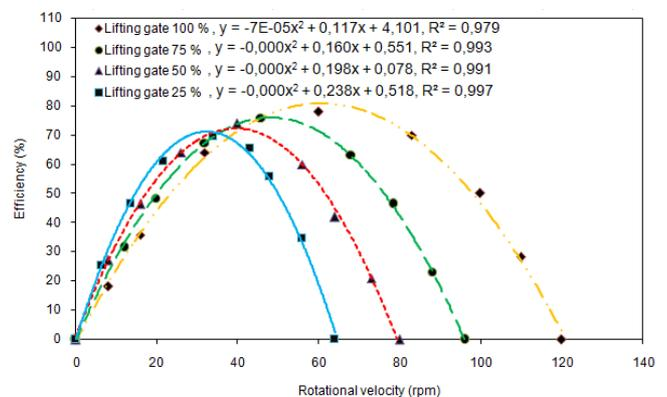
Fig. 17 Curve effect of rotational variations on W2KDS efficiency
