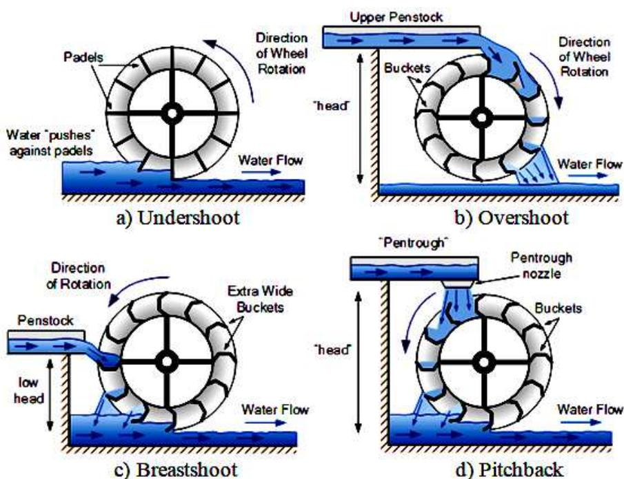
Fig. 1 Four types of water wheels
