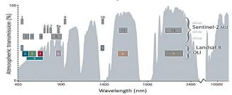
Fig. 3 Comparison between OLI Landsat-8 and MSI sentinel-2 spectral bands
