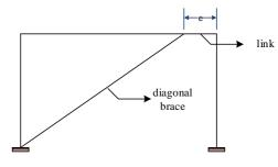
Fig. 1. Eccentrically Braced Frame
