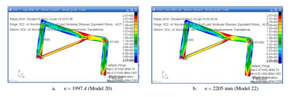
Fig. 12 . Numerical failure mode for the intermediate link (bending dominant)
