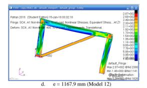
Fig. 10. The numerical failure mode for short link
