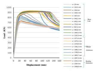
Fig. 8. Load - displacement relationship for various link's length
