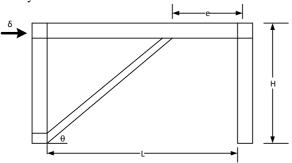
Fig. 3. Structure model- a D-Braced Eccentrically Braced Frame
