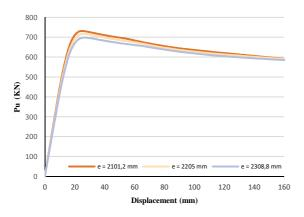
Fig 7. Load – displacement relationship for intermediate link (2.6 Mp/Vp < e < 5 Mp/Vp)
