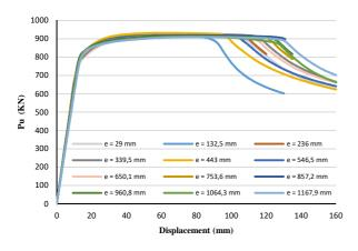
Fig. 5. Load - displacement relationship for shear link
