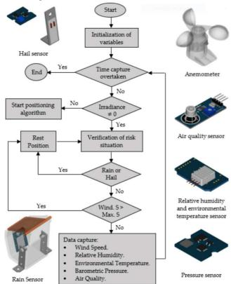
Fig. 6. Arduino Weather Station Sensor and Logic [51]
