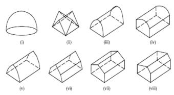
Fig. 1. Classification of greenhouses based on the shape of the roof [16]
