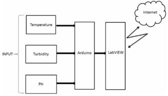
Fig. 5. Water Quality Monitoring Architecture [49]
