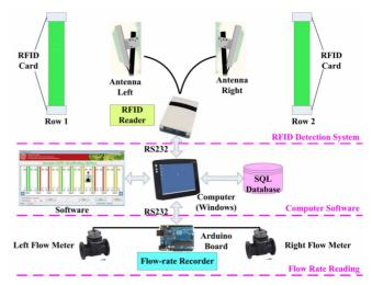
Fig. 7. Design of RFID-based Monitoring System [54]
