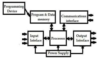
Fig. 2. PLC Based Process Control [27]
