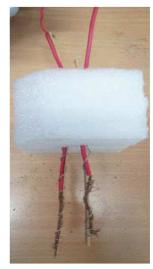
Fig. 3. Homemade Soil Moisture Sensor [39]
