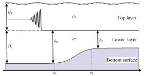
Fig. 1 Schematic illustration of an internal undular bore propagates over a varying slope
