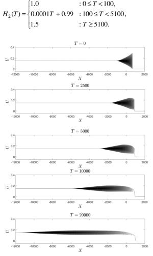
Fig. 7 2D plot of an undular bore with a leading KdV-type solitary wave at the leading edge propagating over a slowly decreasing slope where  $h_1 = H_1$
