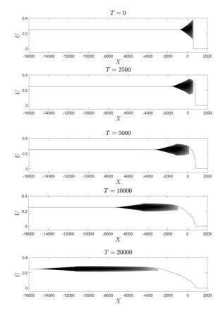
Fig. 10 2D plot of an undular bore with a leading table-top solitary wave at the leading edge propagating over a slowly decreasing slope where  $h_1 > H_1$
