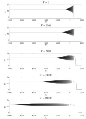
Fig. 6 2D plot of an undular bore with a leading table-top solitary wave at the leading edge propagating over a slowly decreasing slope where  $h_1 < H_1$
