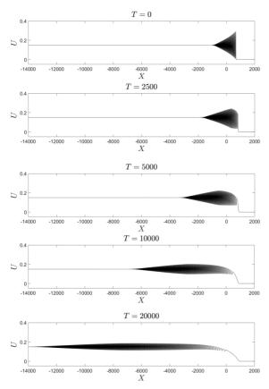
Fig. 9 2D plot of an undular bore with a leading KdV-type solitary wave at the leading edge evolving over a slowly decreasing slope where  $h_1 > H_1$
