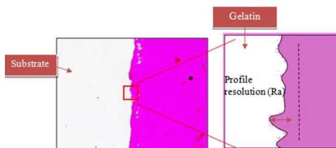
Fig. 2 Method for determining resolution by measuring average straightness on the edge of the patterned gelatin on a glass plate
