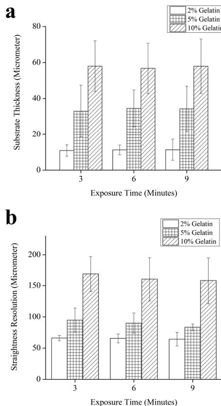
Fig. 5 (a) Thickness of the gelatin substrate at various concentration and exposure time; and (b) resolution of patterned gelatin at different concentration and exposure time
