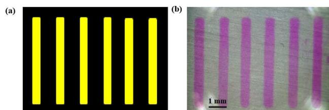
Fig. 3 The pattern of gelatin substrate in a computer screen; and (b) realized patterned gelatin on a glass plate
