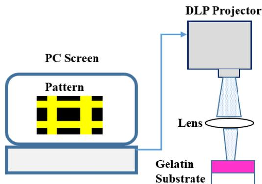
Fig. 1 The experimental setup of photo-patterning of gelatin solution coated onto a glass plate surface with a predetermined pattern using commercial DLP projector
