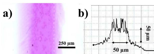
Fig. 4 a) The realized patterned gelatin in 10X magnification, and (b) the result of the contour measurement.
