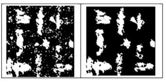
Fig. 7: Bi-level hue image after elimination of small connected areas and hue image after binarized by Huang's thresholding algorithm
